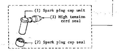
Caution: In case of any engine trouble due to leakage of electricity from the spark plug cap (mis-firing of the engine), the plug cap should be charged to the new type and at the same time an "O" ring should be fixed to the cylinder head cover.
